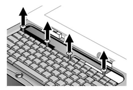
Figure 2-7. Loosening the Keyboard Retaining Screws
