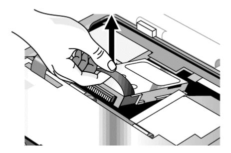
Figure 2-9. Removing the Hard Disk Drive
