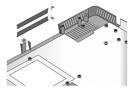
Figure 2-25. Installing the PCMCIA Doors
