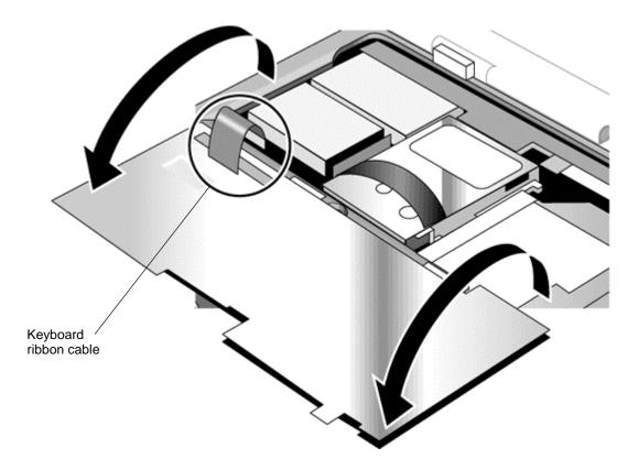
Figure 2-8. Disconnecting the Keyboard Cable
