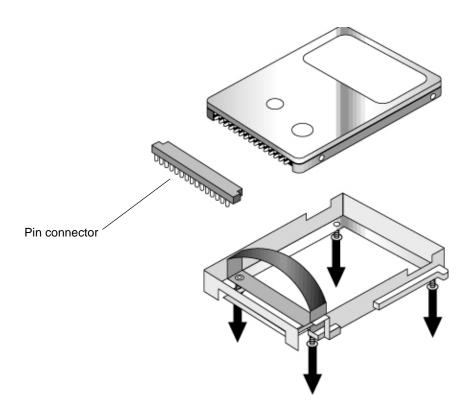
Figure 2-10. Removing the Hard Disk Carrier
