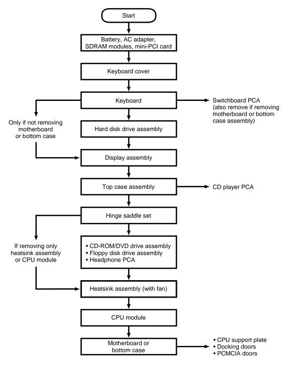
Figure 2-1. Disassembly Flow
