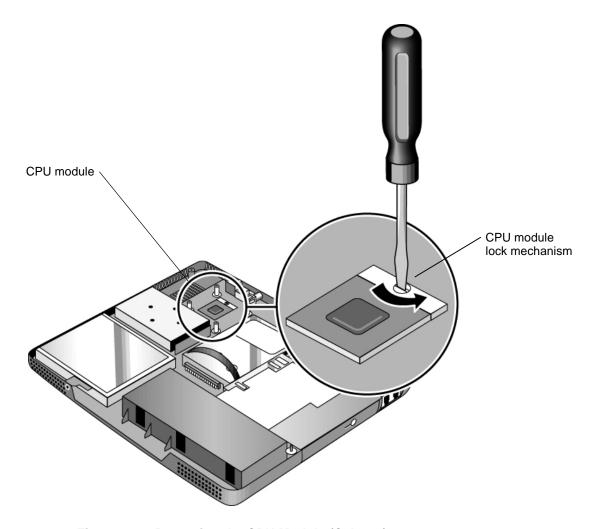
Figure 2-20. Removing the CPU Module (Celeron)
