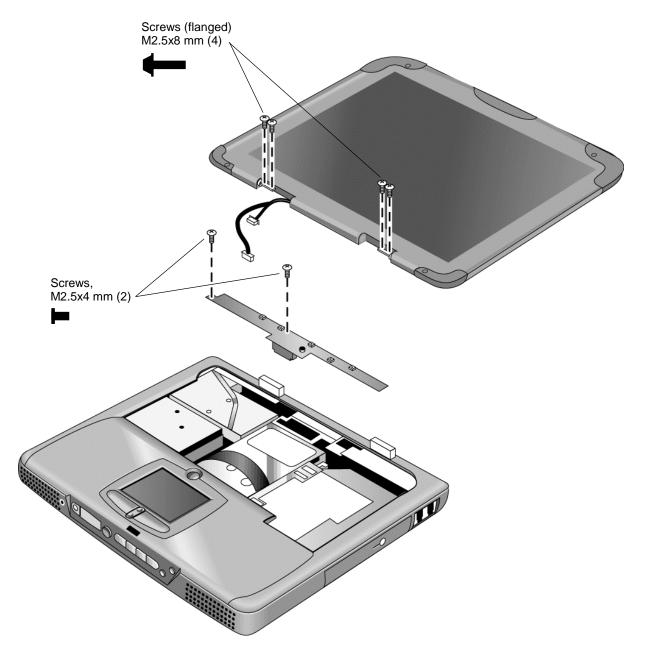
Figure 2-11. Removing the Display
