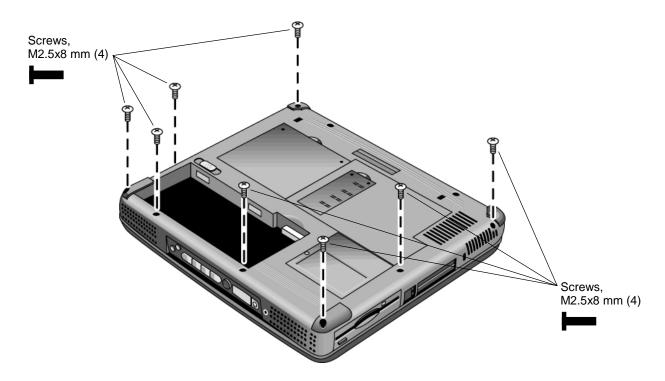
Figure 2-13. Removing the Top Case Retaining Screws
