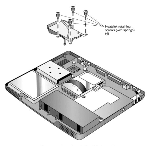
Figure 2-18. Removing the Heatsink Assembly
