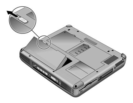
Figure 2-2. Removing the Battery
