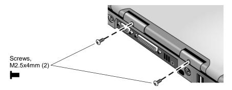
Figure 2-5. Removing the Keyboard Cover Retaining Screws
