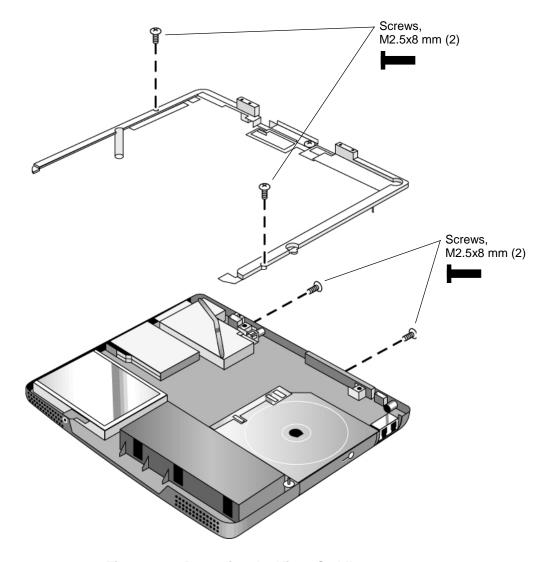
Figure 2-17. Removing the Hinge Saddle
