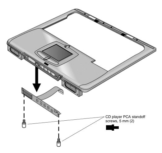
Figure 2-15. Removing the CD Player PCA
