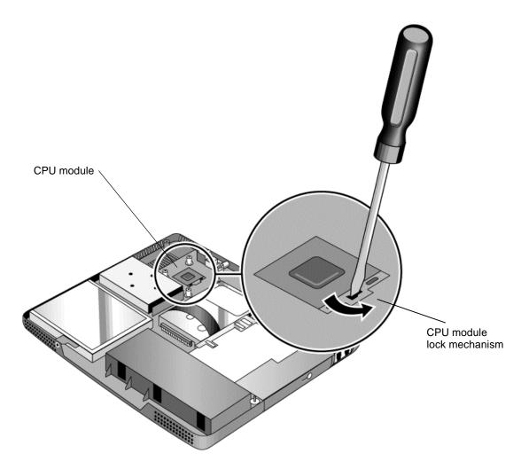
Figure 2-19. Removing the CPU Module (Pentium)
