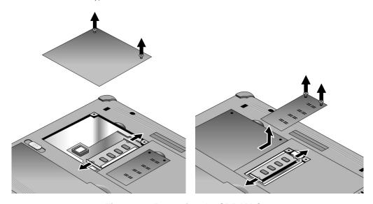
Figure 2-3. Removing the SDRAM Covers
