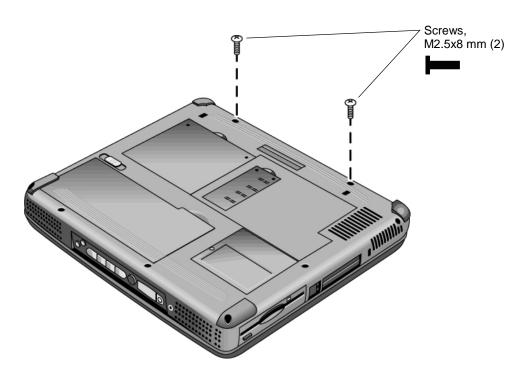
Figure 2-16. Removing the Hinge Saddle Retaining Screws
