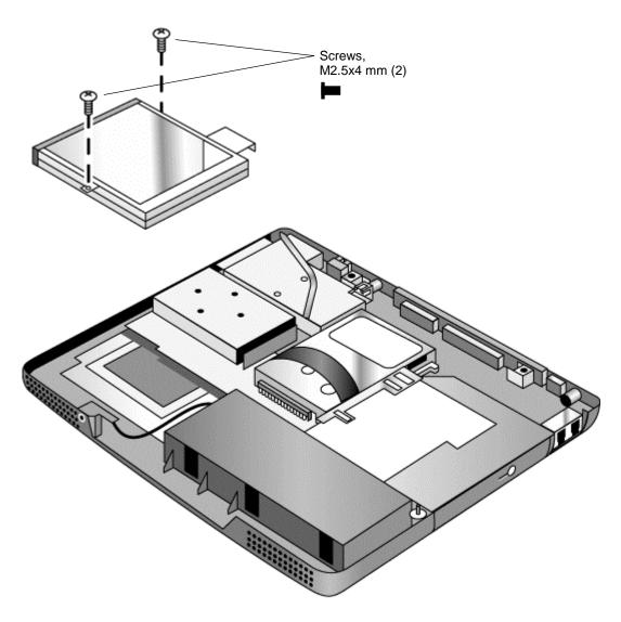
Figure 2-21. Removing the Floppy Disk Drive
