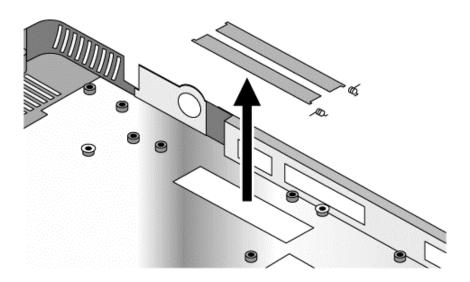
Figure 2-24. Installing Docking Doors
