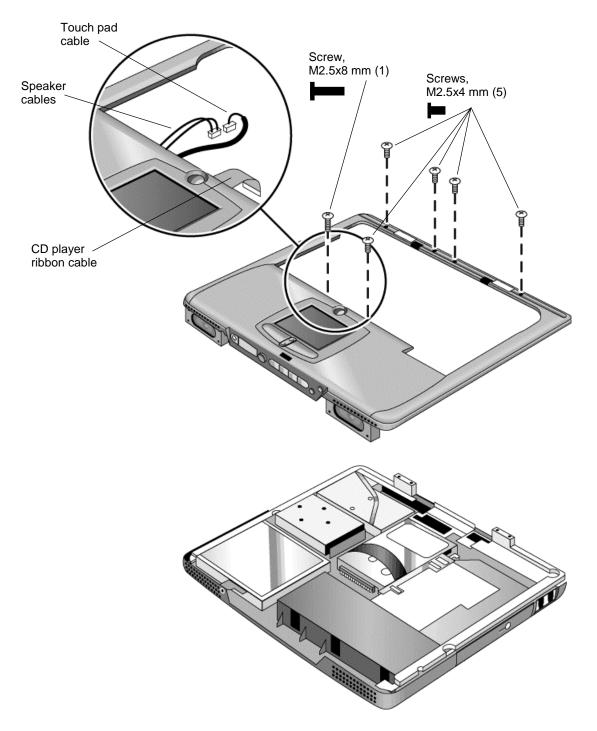
Figure 2-14. Removing the Top Case
