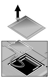
Figure 2-4. Removing the Mini-PCI PCA
