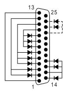
Figure 3-3. Parallel Loopback Connector
