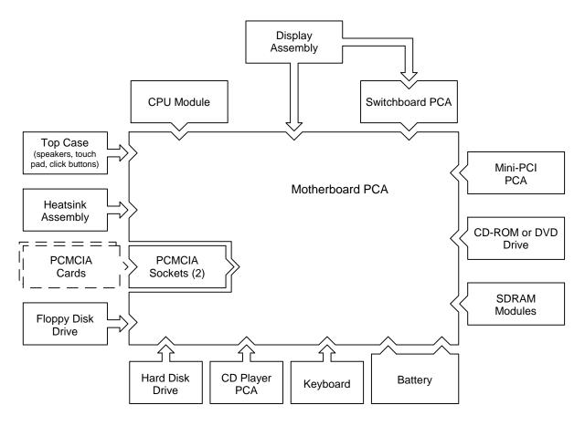
Figure 1-8. Replaceable Module Diagram
