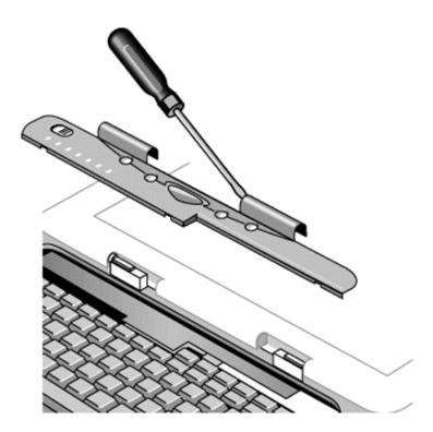
Figure 2-6. Removing the Keyboard Cover
