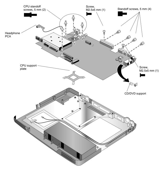
Figure 2-23. Removing the Motherboard
