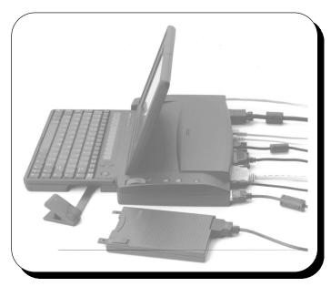
The Enhanced Port Replicator Accessory consists of no field replaceable components. If any component of the dock is defective, the entire unit must be replaced.
