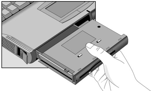
5. With the latch in the open position, slide the battery into the OmniBook until flush with the unit.
