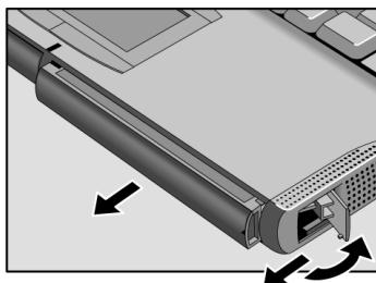
5. Grasp the underside of the battery firmly and pull out.
