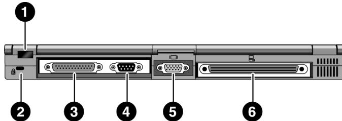
1. Infrared port. Windows NT 4.0 does not support infrared communication.
