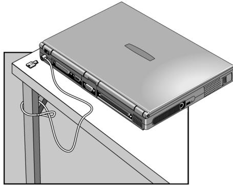
2. Loop the cable to create a slip knot around the stationary object—make sure it can't slip off
