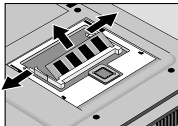
5. Pull the board out of the connector.
