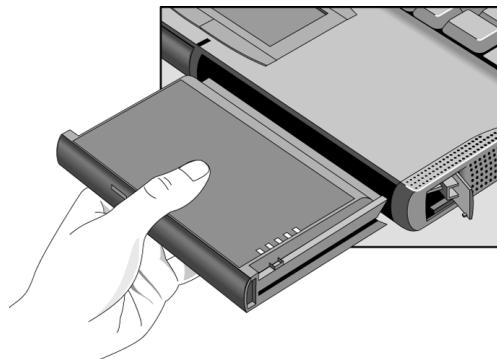
6. With the latch in the open position, slide the charged battery into the OmniBook until it is flush with the unit.
