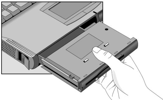
5. With the latch in the open position, slide the new plug-in module into the OmniBook until flush with the unit.
