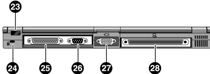
23. Infrared port. Windows NT 4.0 does not support infrared communication.
