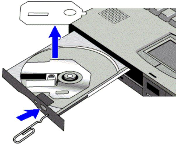
3. Place the CD into the drive (label facing up) and gently press down to seat the CD on the spindle.
