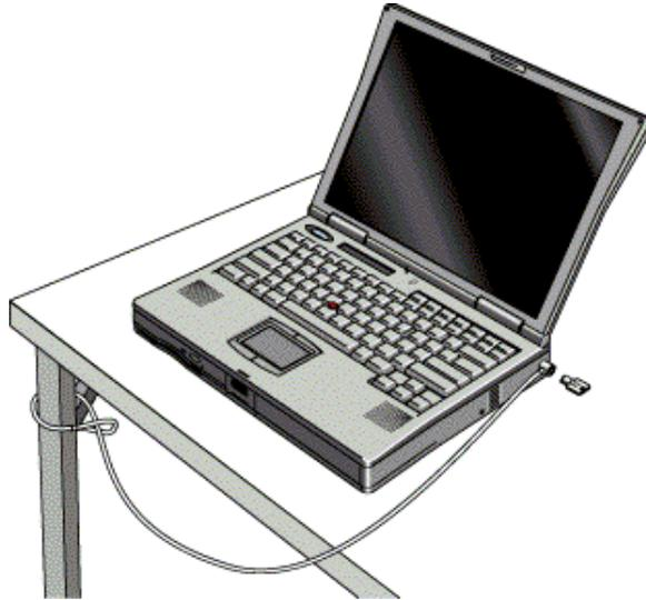
2. Loop the cable to create a slip knot around the stationary object—make sure it can't slip off.
