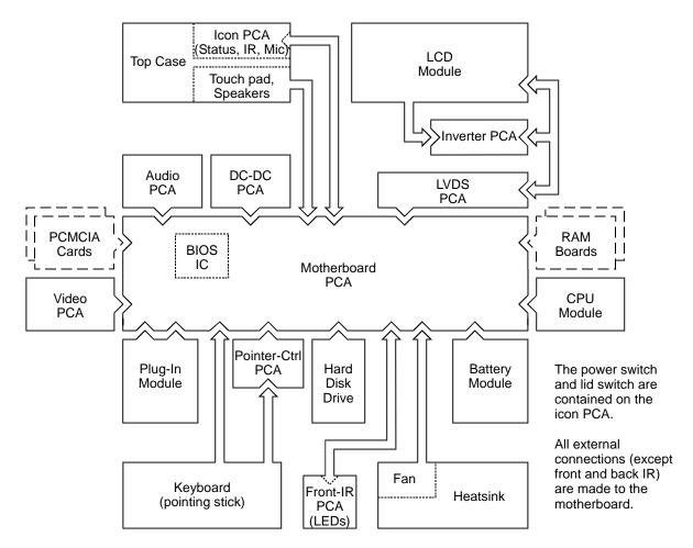
Figure 1-4. Replaceable Module Diagram
