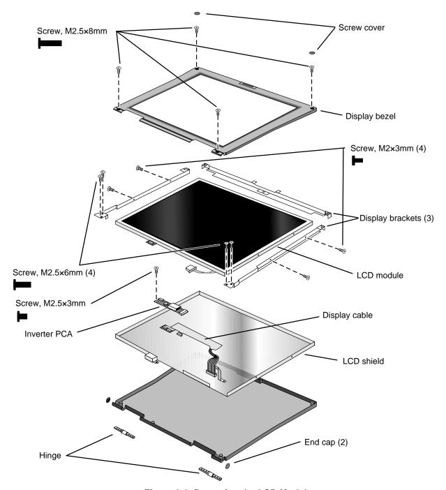
Figure 2-8. Removing the LCD Module
