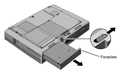
Figure 2-1. Removing the Battery or Module
