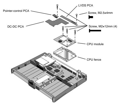
Figure 2-10. Removing the Motherboard (Part 1)
