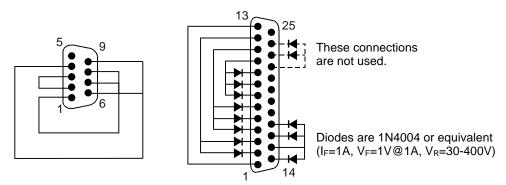
Figure 3-3. Serial and Parallel Loopback Connectors
