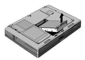
Figure 2-3. Removing the Hard Disk Drive
