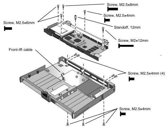
Figure 2-11. Removing the Motherboard (Part 2)
