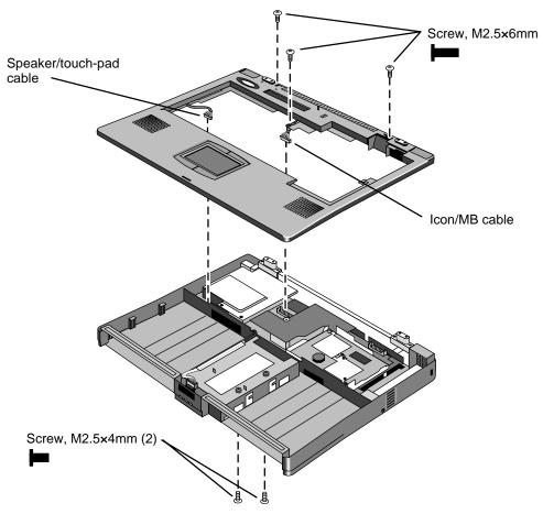
Figure 2-9. Removing the Top Case
