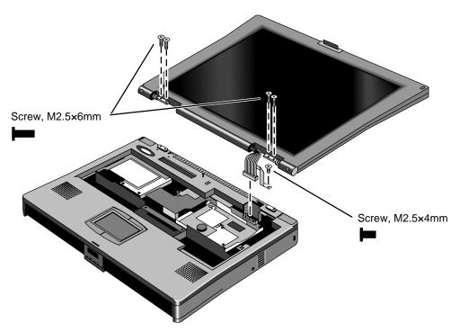
Figure 2-7. Removing the Display Assembly
