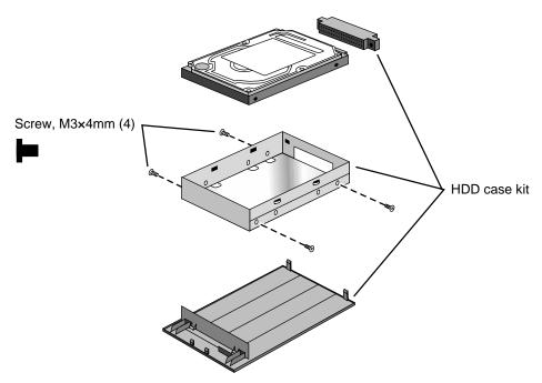
Figure 2-4. Installing a Hard Drive in the Case
