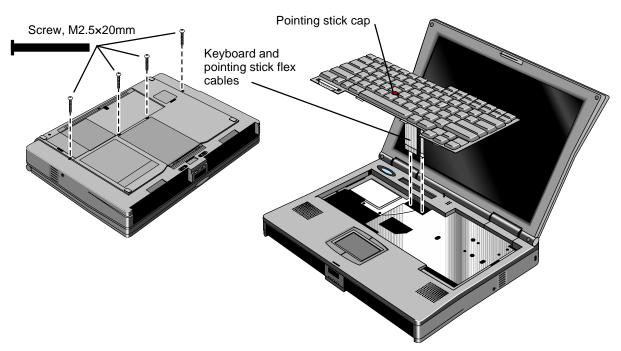
Figure 2-5. Removing the Keyboard
