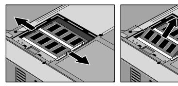
Figure 2-2. Removing a RAM Board
