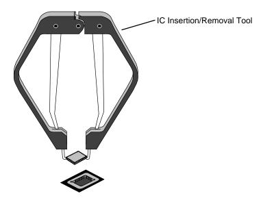
Figure 2-12. Removing the BIOS IC
