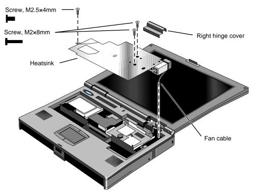
Figure 2-6. Removing the Heatsink
