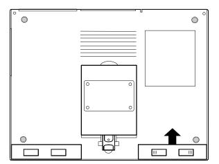
2. Slide the battery module into the empty bay. Carefully press the battery all the way into the compartment. You will hear a click as the locking switches move outward and the module is locked in place.
