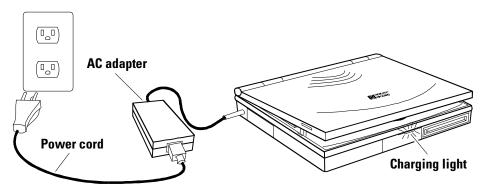
The charging light shows the charging status. An orange color indicates that the adapter is charging your computer's removable battery; the light will turn green when the battery pack is fully charged.
