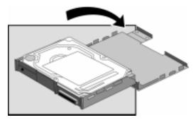
3. Pry out the corner next to the connector, then lift out the connector and hard drive together.
