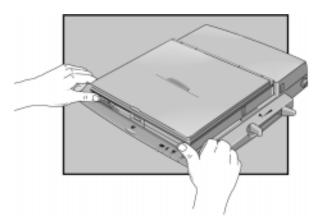
When the OmniBook is properly inserted, the amber wait light turns on. When the OmniBook is ready for use, the green docked light turns on.
