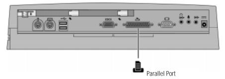
The dock's 25-pin parallel port is a standard enhanced (EPP/ECP) parallel port.
