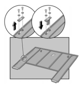
4. Insert the tabs on the back of the tray into the slots in the dock and press down on the front edge of the tray to lock it in place.
