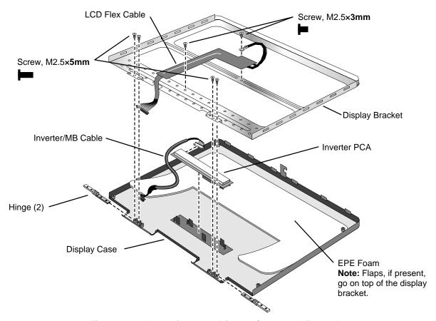
Figure 2-14. Removing a 13" Display Case and Display Bracket
