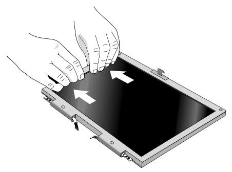
Figure 2-10. Removing the Display Bezel
