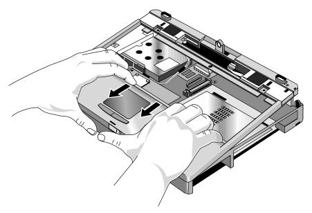
Figure 2-19. Removing the Top Case
