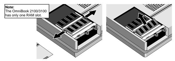
Figure 2-6. Removing a RAM Board
