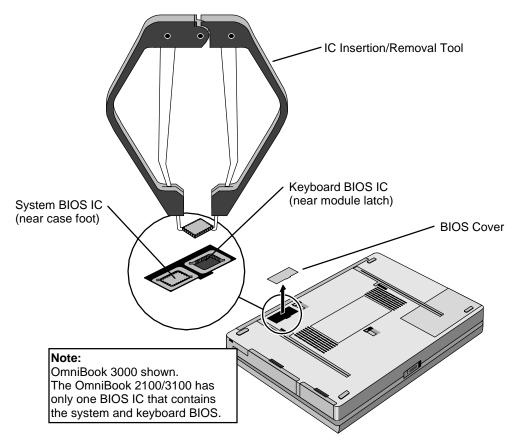
Figure 2-23. Removing a BIOS IC
