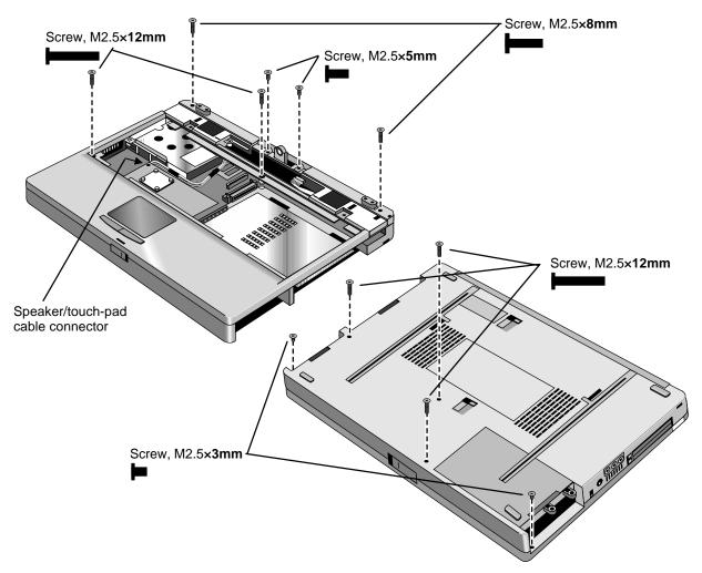
Figure 2-18. Removing the Case Screws
