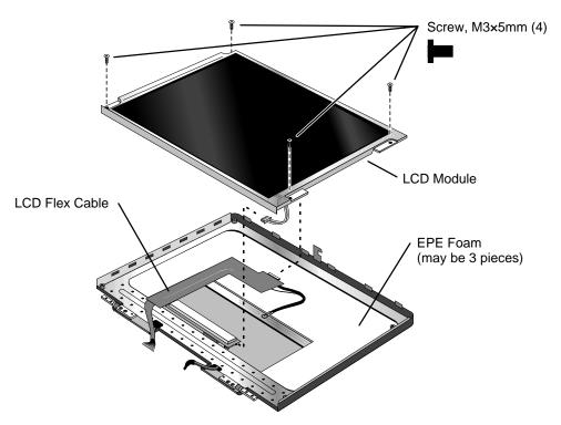
Figure 2-12. Removing the 13" LCD Module
