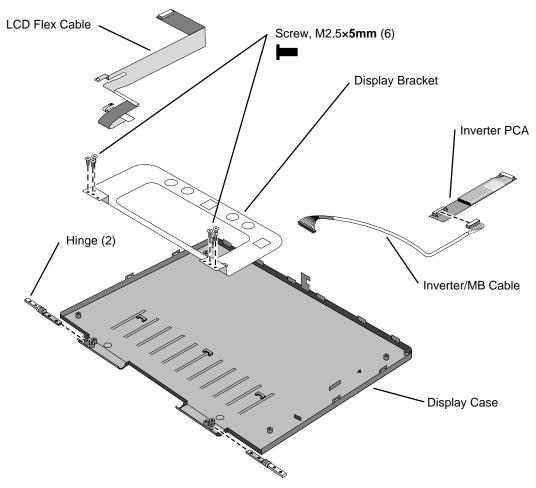
Figure 2-13. Removing a 12" Display Case and Display Bracket
