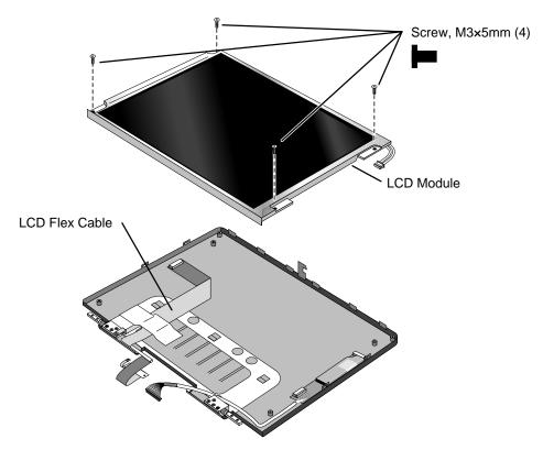
Figure 2-11. Removing the 12" LCD Module
