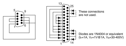
Figure 3-3. Serial and Parallel Loopback Connectors
