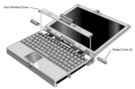
Figure 2-15. Removing the Hinge Covers and Icon Window Cover
