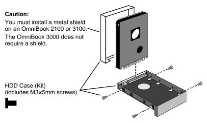
Figure 2-4. Installing a Hard Drive in the Case
