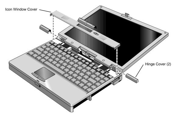
Figure 2-7. Removing the Hinge Covers and Icon Window Cover
