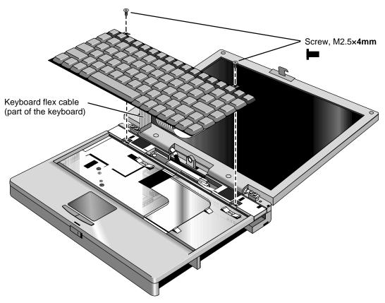
Figure 2-16. Removing the Keyboard
