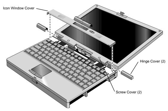
Figure 2-9. Removing the Hinge Covers and Icon Window Cover
