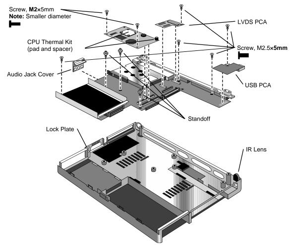
Figure 2-21. Removing the Motherboard
