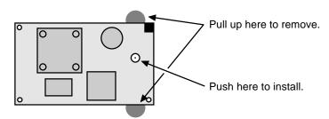
Figure 2-20. Removing and Installing the CPU Module
