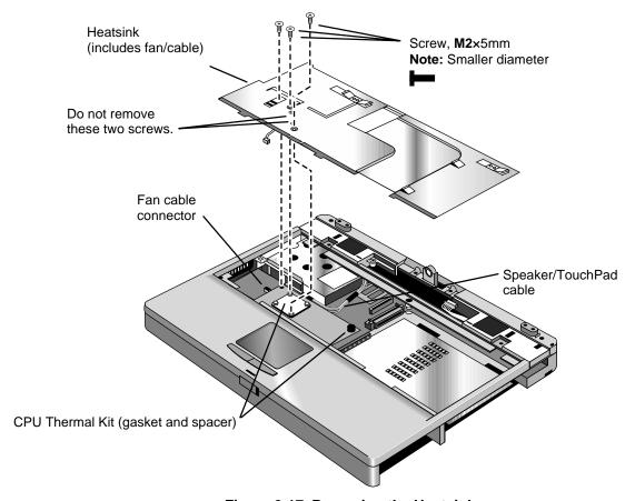
Figure 2-17. Removing the Heatsink
