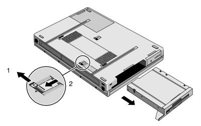
Figure 2-2. Removing a Plug-In Module
