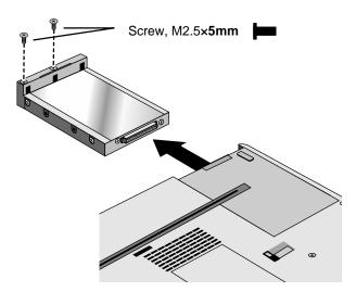
Figure 2-3. Removing the Hard Drive
