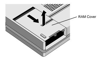
Figure 2-5. Removing the RAM Cover
