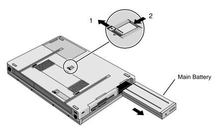
Figure 2-1. Removing the Main Battery
