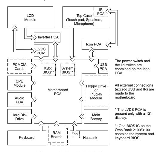
Figure 1-4. Replaceable Module Diagram
