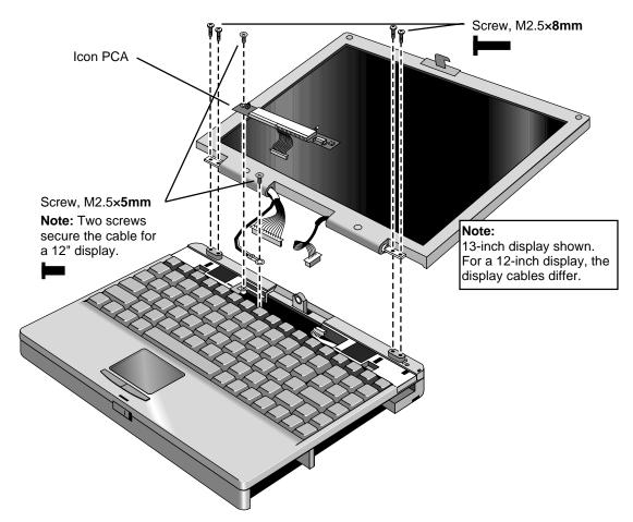
Figure 2-8. Removing the Icon PCA and Display Assembly
