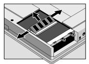
7. Insert the hard disk drive and battery.
