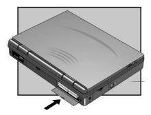
4. While firmly holding the OmniBook against the docking pins, slide the docking lever back and release, then press the blue On/Suspend button.
